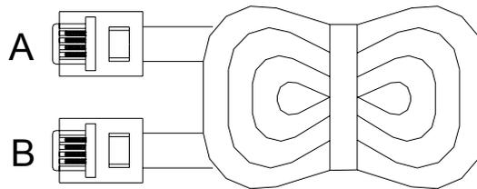
The A and B connectors on the rear of the converter are RJ-11 connectors. These connectors are wired identically. The RJ-11 connectors have six positions, two of which are wiring, The Converter uses the center two pins. The pin out assignment for these connectors is presented below.
