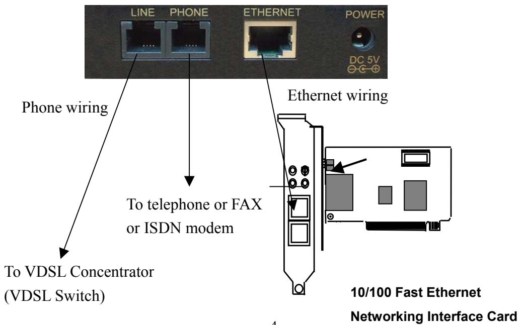
1. The RJ-11 port supports 10 Mbps connections. When inserting a RJ-11 plug, be sure the tab on the plug clicks into position to ensure that it is properly seated.
